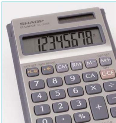
Liquid crystal display used in a calculator
