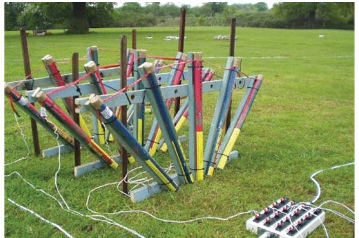
*Electrical firing systems for fireworks displays*
