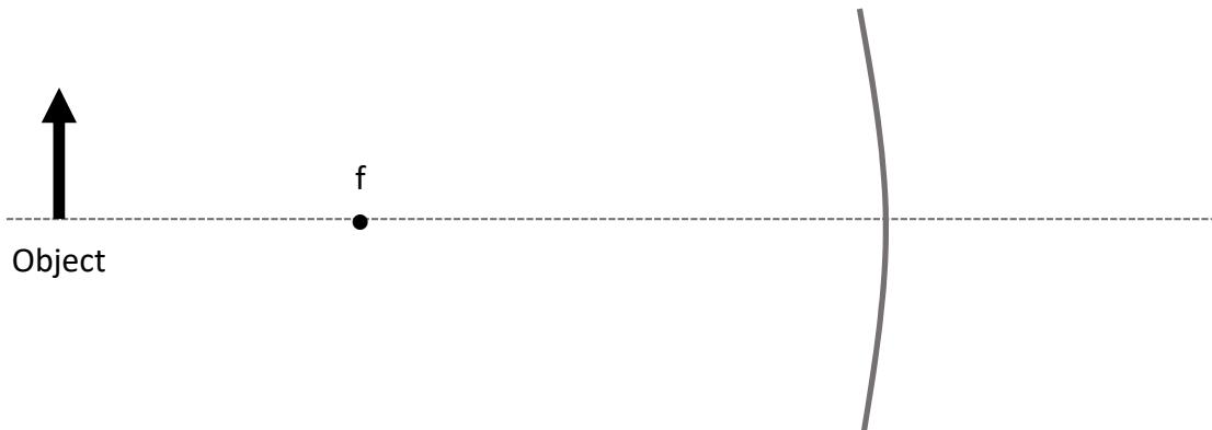
An object of height 2 cm is placed 17 cm in front of a concave mirror.
