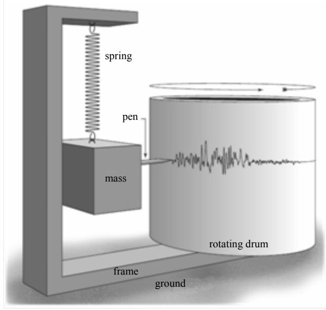
A seismometer consists of a sensor that detects ground motion, attached to a recording system. A seismometer that is sensitive to up-down motions of the ground, as caused by an earthquake, can be understood by visualising a mass hanging on a spring as shown in the diagram. The frame and the drum move up and down as the seismic wave passes by, but the mass remains stationary.
