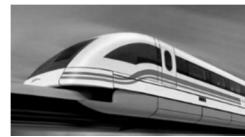
**Part (c) Magnetically levitated trains (known as maglev trains) use magnets under their carriages to float above the magnetic tracks.**
