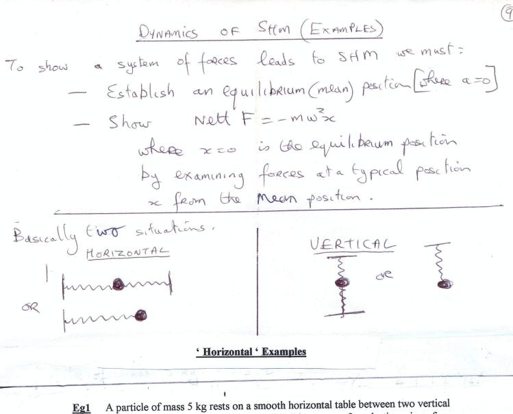
Eg1 A particle of mass 5 kg rests on a smooth horizontal table between two vertical walls, 7 m apart. It is attached to the left hand wall by means of an elastic spring of natural length 1 m and elastic constant 12 N/m and to the right hand wall by means of an elastic string of natural length 1 m and elastic constant 8 N/m. The particle is released from rest 1.5m from the right hand wall.
