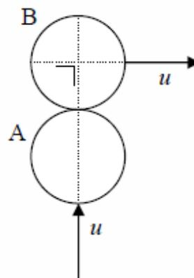
The line of centres at the instant of impact is perpendicular to the direction of motion of sphere B.
