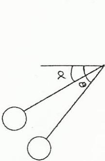
Gain in kinetic energy = Loss in potential energy
