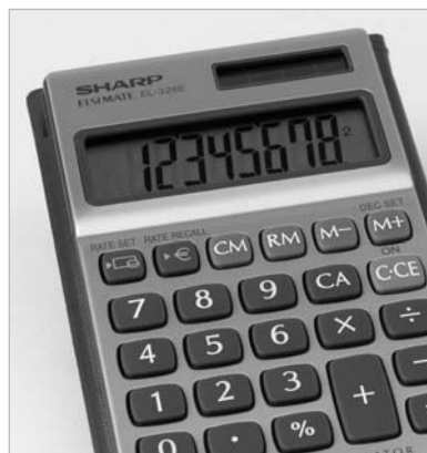
Liquid crystal display used in a calculator Reproduced with kind permission of Sharp Consumer Electronics.
