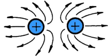
(v) Mark on your diagram a place where the electric field strength is zero.
