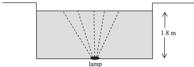
A lamp is located centrally at the bottom of a large swimming pool, 1.8 m deep.
