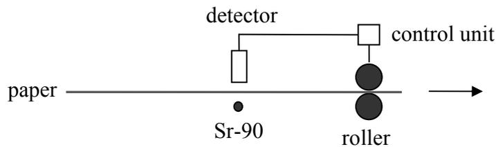
The radioisotope used is Sr-90 and it emits beta-particles, which are recorded by the detector. The output from the detector adjusts the gap between the rollers, so that the paper is of uniform thickness.
