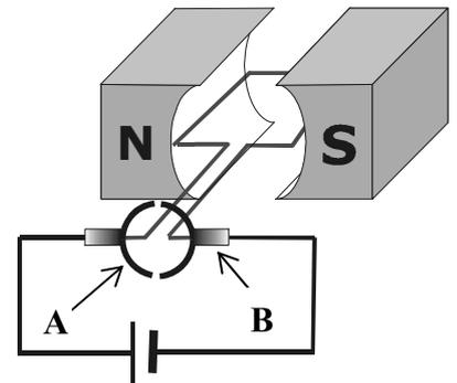
If the motor jammed, a larger current than normal would flow through the motor.
