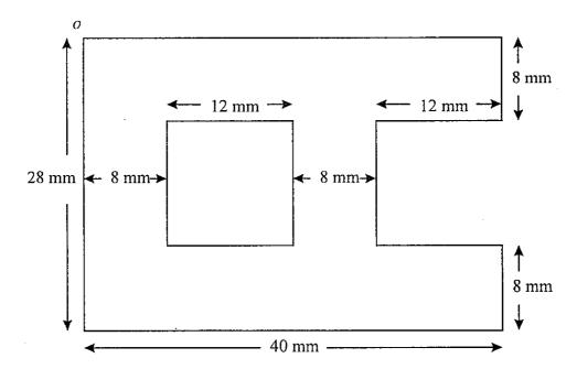
Calculate the distance from the point o to the centre of gravity of the remaining piece, correct to one place of decimals.
