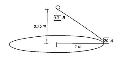
Show, on separate diagrams, all the forces acting on A and B.
