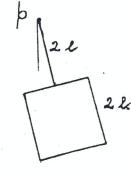
(ii) A thin uniform rod of length 21 and of mass m is attached to the mid point of the rim of the square. Find the moment of inertia of the system about an axis through p perpendicular to the common plane of the lamina and rod. [See Tables, P.40].
